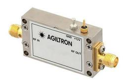
The LNAM series low noise amplifiers are designed to drive lithium niobate modulators. These amplifiers enhance the RF input signal to reach modulator's Vp at high frequencies. They use 50 Ohm SMA connectors and operate within a frequency range of 50 kHz to 50 GHz.
